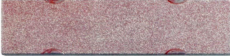
Figure 1: Almen strip aspect, previously painted, after shot-peening treatment.
